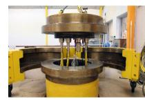
Hydrostatic pressure testing
