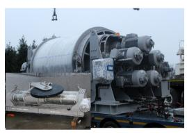
RA winch with AHC and speed of 3m/s
